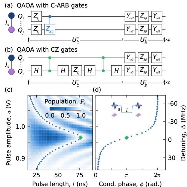
FIG. 1. (a) Quantum circuit of a layer  $q$  of QAOA for the two-qubit subspace  $|Q_i Q_j\rangle$ , using the controlled arbitrary-phase gate (blue) to rotate the  $|11\rangle$  state by an angle  $2\Gamma_{ij}$  where  $\Gamma_{ij} = 2\gamma_q J_{ij}$ . (b) A QAOA layer with the phase-separation unitary  $U_C^{ij}$  decomposed into CZ gates (green) and additional Hadamard gates and single-qubit Z-gates. (c) Excited-state
